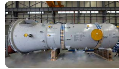
- Cracked Gas Chiller Drum
