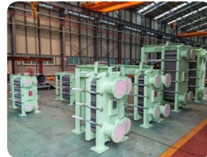
- Plate heat Exchanger
