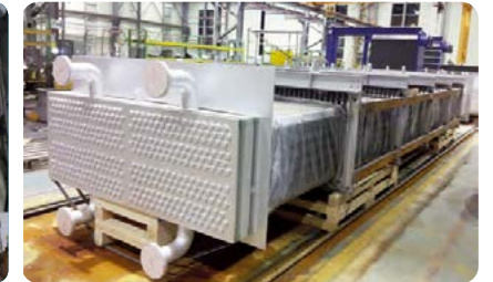
- Steam Coil Air Heater
