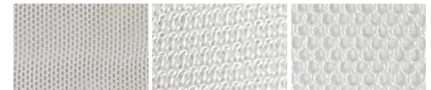
Material Polyamide(Nylon) Weaving type Knit(Single layer)
