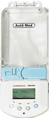
2) AutoMed 3300 Reusable electronic PCA with its compartment for disposable set mounted on
