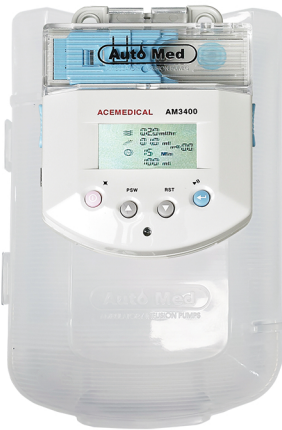
3) AutoMed 3400 Reusable electronic PCA compatible with other
