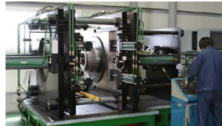
▲ Automatic Hydraulic Forming Machine (Max. 750mm)
