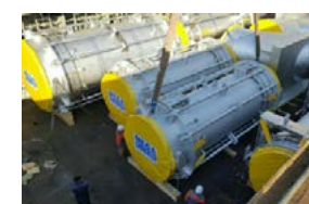
▲ Various Expansion Joints View
