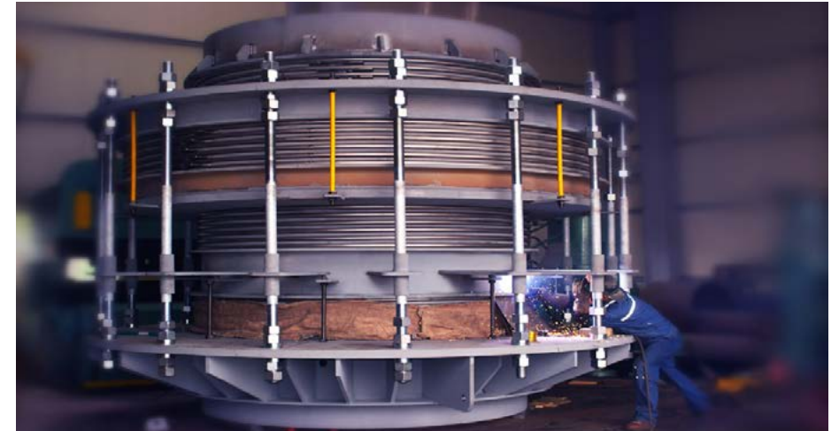
In-line Pressure Balanced Expansion Joint for SHUWEIHAT S2 IWPP, ABU DHABI UAE
